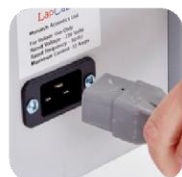
IEC power cable into the mains.
