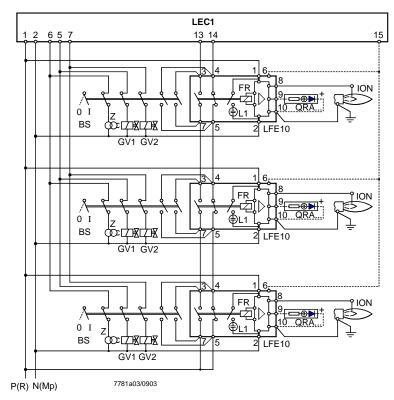
Like with dual-supervision, the control contacts of the flame relays of all flame safeguards must be connected in series when using multi-flame supervision.
