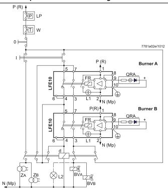
With this type of supervision, too, the burner can be started only if the flame detector or flame simulation test has been successful. This means that **neither** of the 2 flame safeguards may detect a flame signal during burner off times. When the burner is started up, the detector test will automatically be interrupted.
