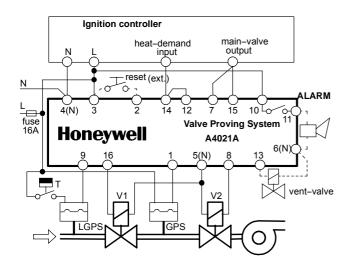
Fig. 10. Wiring diagram for 2-valve configuration pre-configuration
