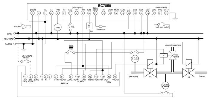
Fig. 14. Wiring diagram A4021A- EC7850 pre-configuration: intermittent pilot and vent-valve to open atmosphere
