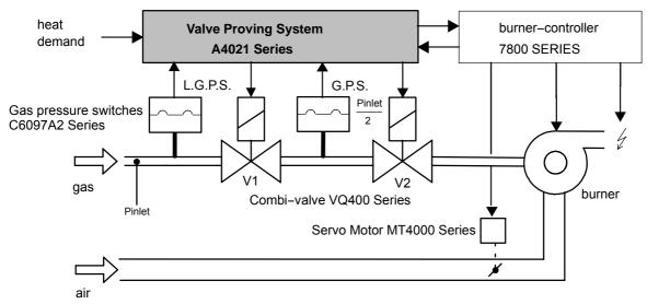
Fig. 4. System set-up .
