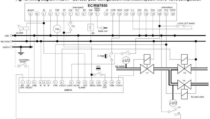
Fig. 17. Wiring diagram A4021A- EC7850 with by-pass valve, post configuration
