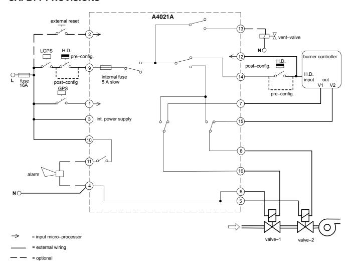
Fig. 9. Simplified internal schematic and wiring diagram pre- and post-test configuration.
