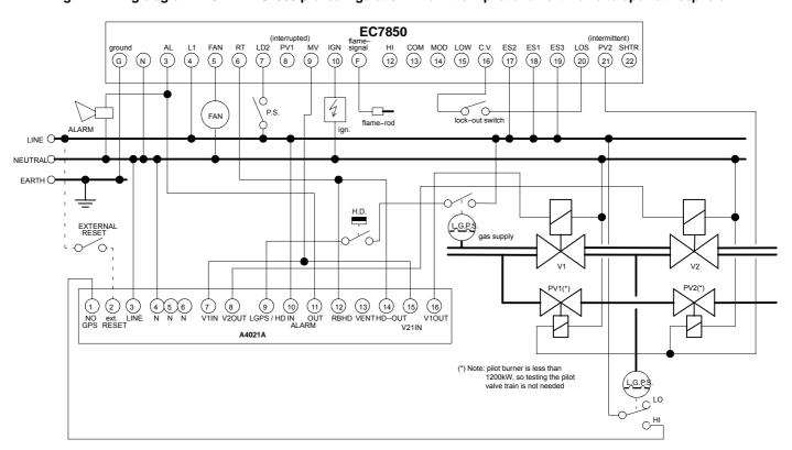
Fig. 15. Wiring diagram A4021A - EC7850: pre-configuration, intermittent pilot, 4-valve configuration
