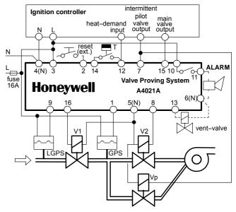
Fig. 13. Wiring diagram 3-valve configuration (post-configuration)
