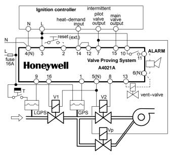
Fig. 12. wiring diagram 3-valve configuration (pre-configuration)
