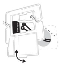
**C)** Attach the thermostat to the wallplate when finished.
