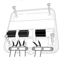
C) Replace the cover Locate the hinges at the top of the cover and wall plate, close the cover and secure with the
