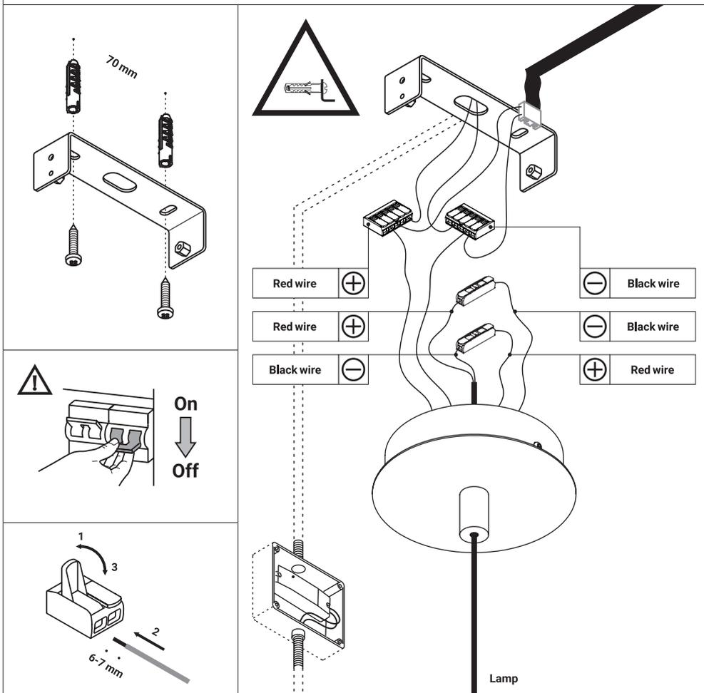
Example of connection with Endless and power kit with plug
