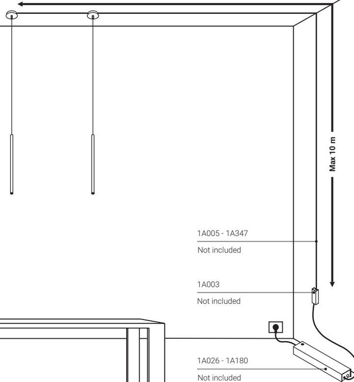
Example of connection with Endless and remote driver
